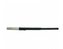
Sonde IP67 étanche multi-usage étanche à l' eau - 80 à + 200 ° C. Temperature probes marked II3G Ex ec IIC T3 Gc and II3D Ex tc IIIC T60 °C... 230 °C Dc can be used in potentially explosive atmospheres - equipment group II, zone 2 and zone 22.
