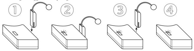
The procedure is identical with the above procedure for switching ON. If indication yellow LED does not light up to 1 second after plugging the magnet, it is necessary to unplug magnet and repeat the procedure.
