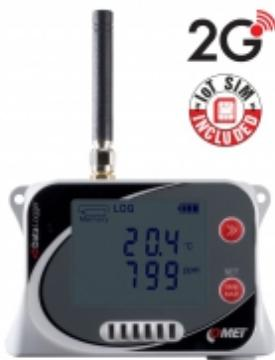
IoT Wireless Datalogger kit with built-in GSM modem and Flat Rate SIM Card allows the instant connection to the COMET Cloud.
