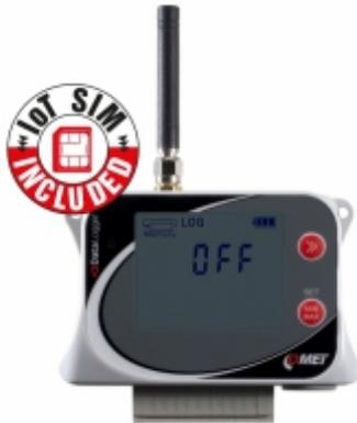
IoT Wireless Datalogger kit with built-in GSM modem and Flat Rate SIM Card allows the instant connection to the COMET Cloud. IoT Datalogger is designed to record from four binary inputs or from two pulse and two binary inputs. In case of exceeded set limits e-mail is sent from the [COMET Cloud](#).
