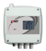
The W0941 sensor with LoRaWAN network output measures temperature from four external Pt1000 probes on the cable and can be installed directly in the measured environment thanks to its IP65-rated enclosure. LoRa devices are powered by a replaceable battery with a lifespan of up to 10 years (3 years standard).
