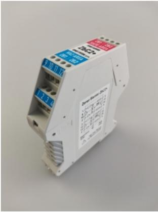
**The Zener barrier ZbC2+ is a certified intrinsically safe interface .** It is used to connect a certified intrinsically safe device located in a potentially explosive atmosphere (Hazardous area) to a non-certified device that is in a safe area.
