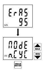
Clearing procedure is in progress. The duration is indicated by displaying of already cleared memory in % (digits 0 to 100).
