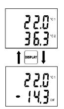
Temperature T1 of channel 1 is displayed on the upper LCD line in °C, temperature T2 of channel 2 is displayed on the lower LCD line in °C.
