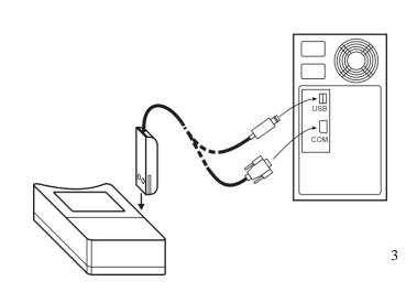
connection via RS232 serial port it is necessary to use COM ADAPTER, for connection via USB port it is necessary to use USB ADAPTER. Connect adapter connector to proper computer port and plug the adapter to the guide slots on the side of logger.
