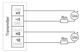
Loop resistance value Rc = Rm + resistance of wires shall fulfill the condition  $Rc[\Omega] < 40 \times Uss[V] - 360$ .
