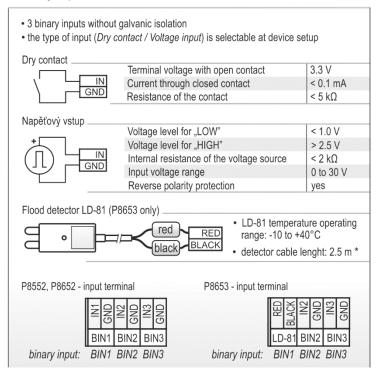
\* the detector cable can't be extended
