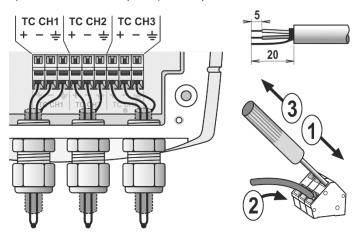
Finally, tighten the cable glands of the connected thermocouple probes to secure and seal the cables. Cables / wires with a diameter of less than 2 mm cannot be sealed in the gland. Also, do not use probes with a braided jacket (glass or metal fabric) in applications where you require the device to be waterproof. Insert attached plug into unused cable glands to seal the device.
