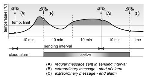
No even a short-term alarm (i.e. with a duration of 1 to 10 min) will not be lost – the information will be sent no later than 10 min even if the alarm is currently inactive. Device in alarm message sends the maximum value measured during the alarm duration.
