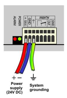
If system is not grounded properly, it is a danger of state, when system floats on variable potential against all other circuitry. It can cause communication dropouts, occasional resets and in extreme case damage of some peripherals. Especially when using pulse power sources (e.g. A1940) it is strongly recommended to ground the system.
