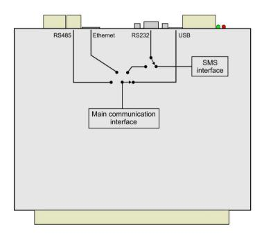
Communication interface can be selected from data logger keyboard or by means of PC program.
