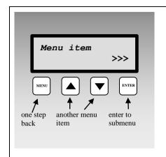
Press MENU key in basic display to enter the data logger Menu. Use , keys to go through all menu items. Press MENU key to leave menu to the basic display.
